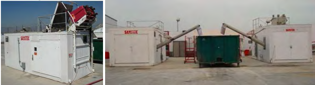
L-R: Cart automatically loaded into the Sanitec system, two Sanitec systems operating side-by-side
